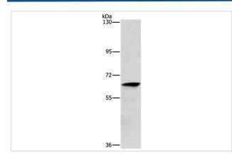
Gel: 10%SDS-PAGE Lysates (from left to right): Human lymphoma tissue Amount of lysate: 40ug per lane Primary antibody: 1/350 dilution Secondary antibody dilution: 1/8000 Exposure time: 30 seconds
