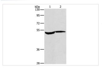
Gel: 8%SDS-PAGE Lysates (from left to right): Human chromaffin cell tumor tissue and A431 cell Amount of lysate: 40ug per lane Primary antibody: 1/350 dilution Secondary antibody dilution: 1/8000 Exposure time: 6 minutes
