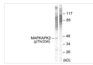
Western blot analysis of extracts from NIH/3T3 cells, using MAPKAPK2 (Phospho-Thr334) antibody #12103. The lane on the right is treated with the synthesized peptide.
