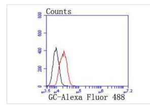
Flow cytometric analysis of HepG2 cells with DBP antibody at 1/50 dilution (red) compared with an unlabelled control (cells without incubation with primary antibody; black). Alexa Fluor 488-conjugated goat anti rabbit IgG was used as the secondary antibody.
