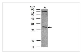
Sample(30 ug of whole cell lysate) A: HeLa S3 12% SDS PAGE Primary antibody diluted at 1: 500
