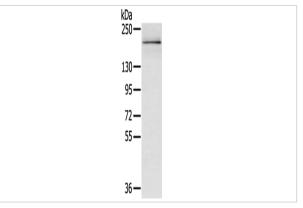
Gel: 6%SDS-PAGE Lysate: 40 µg Lane: Hela cells Primary antibody: 1/200 dilution Secondary antibody: Goat anti rabbit IgG at 1/8000 dilution Exposure time: 5 minutes
