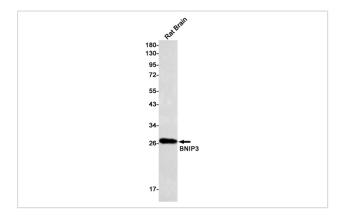
Western blot detection of BNIP3 in Rat Brain lysates using BNIP3 Rabbit mAb(1:500 diluted).Predicted band size:28kDa.Observed band size:28kDa.
