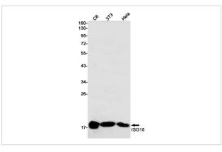
Western blot detection of ISG15 in C6,3T3,Hela cell lysates using ISG15 Rabbit mAb(1:1000 diluted).Predicted band size:18kDa.Observed band size:18kDa.
