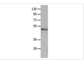
Gel: 10% SDS-PAGE Lysate: 40µg Mouse thymus tissue lysate Primary antibody: 1/900 dilution Secondary antibody: Goat anti Rabbit IgG - H&L (HRP) at 1/5000 dilution Exposure time: 15 seconds
