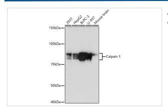
Western blot analysis of extracts of various cell lines, using Calpain 1 antibody.
