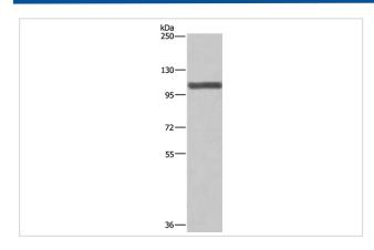
Gel: 6%SDS-PAGE Lysate: 40ug NIH/3T3 cell Primary antibody: 1/275 dilution Secondary antibody dilution: 1/8000
